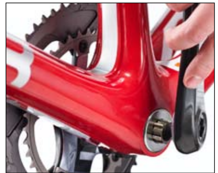
Figure 28. Metal bearing cover in place over the bearing
